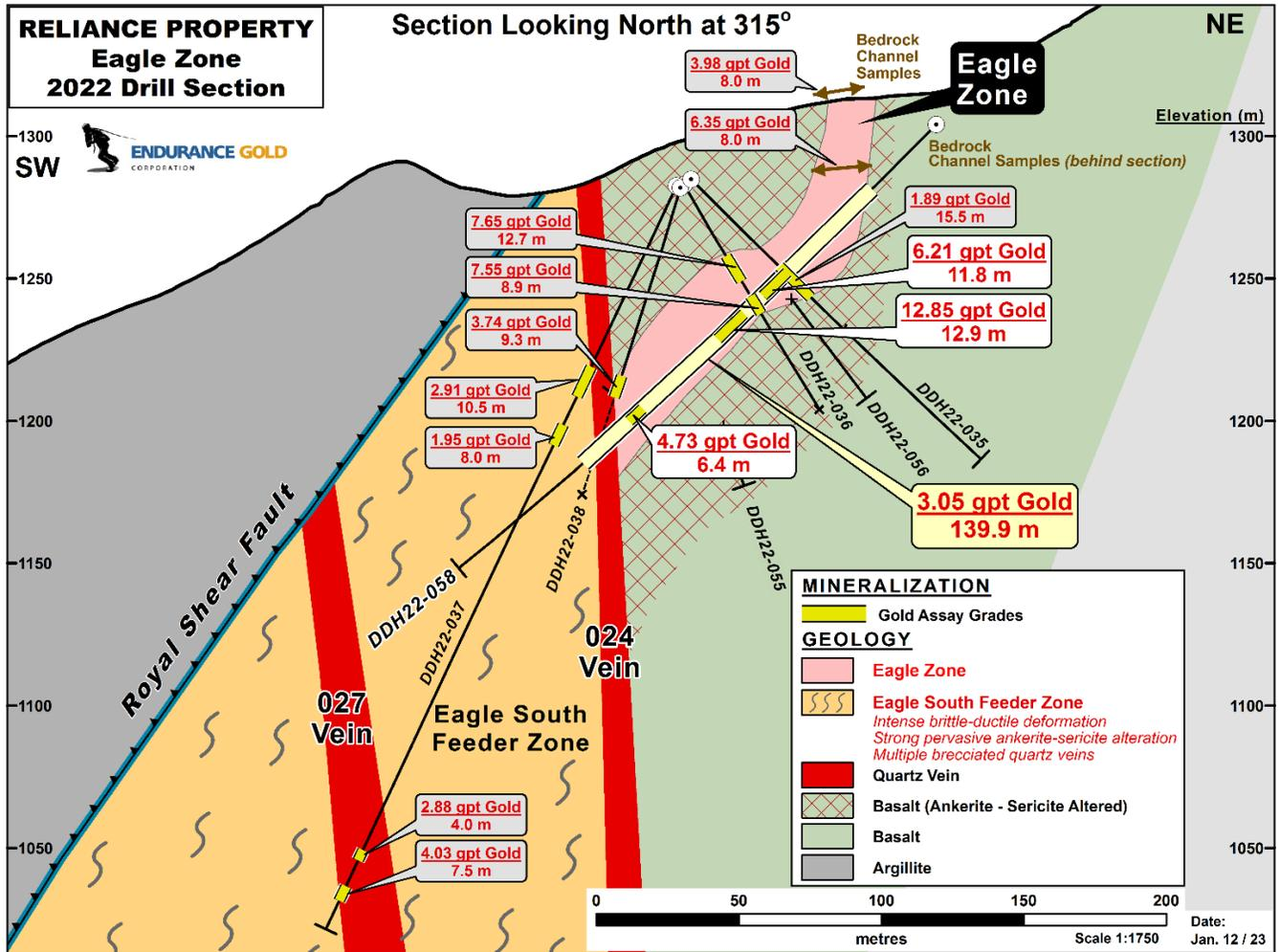
Figure 3: Royal Shear Longitudinal Section
